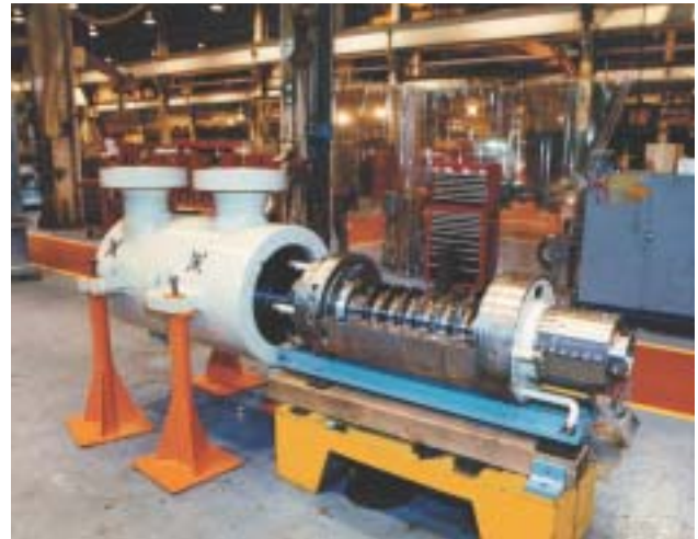
Orion Advantage™ tilting pad bearings are used on this Dresser-Rand "Datum" barrel type process gas compressor. Photo courtesy of Dresser-Rand.
